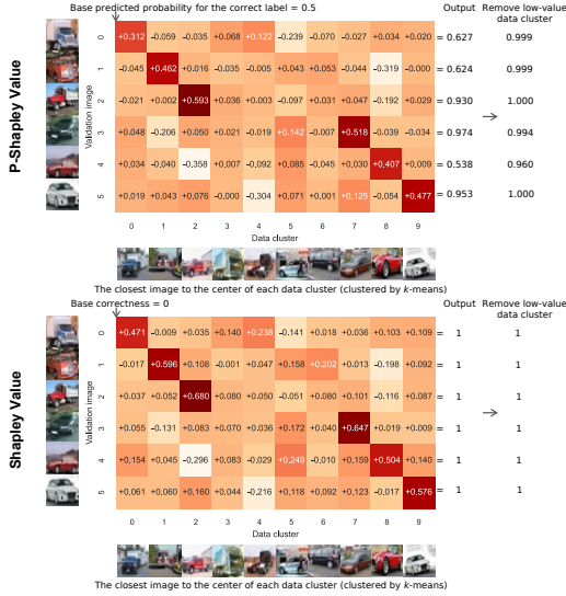
Figure 7: The contribution of each data cluster for the deep learning model’s predicted probability ( resp. prediction correctness) of each validation image on CIFAR-10, and darker colors indicate larger P-Shapley values ( resp. Shapley values).
